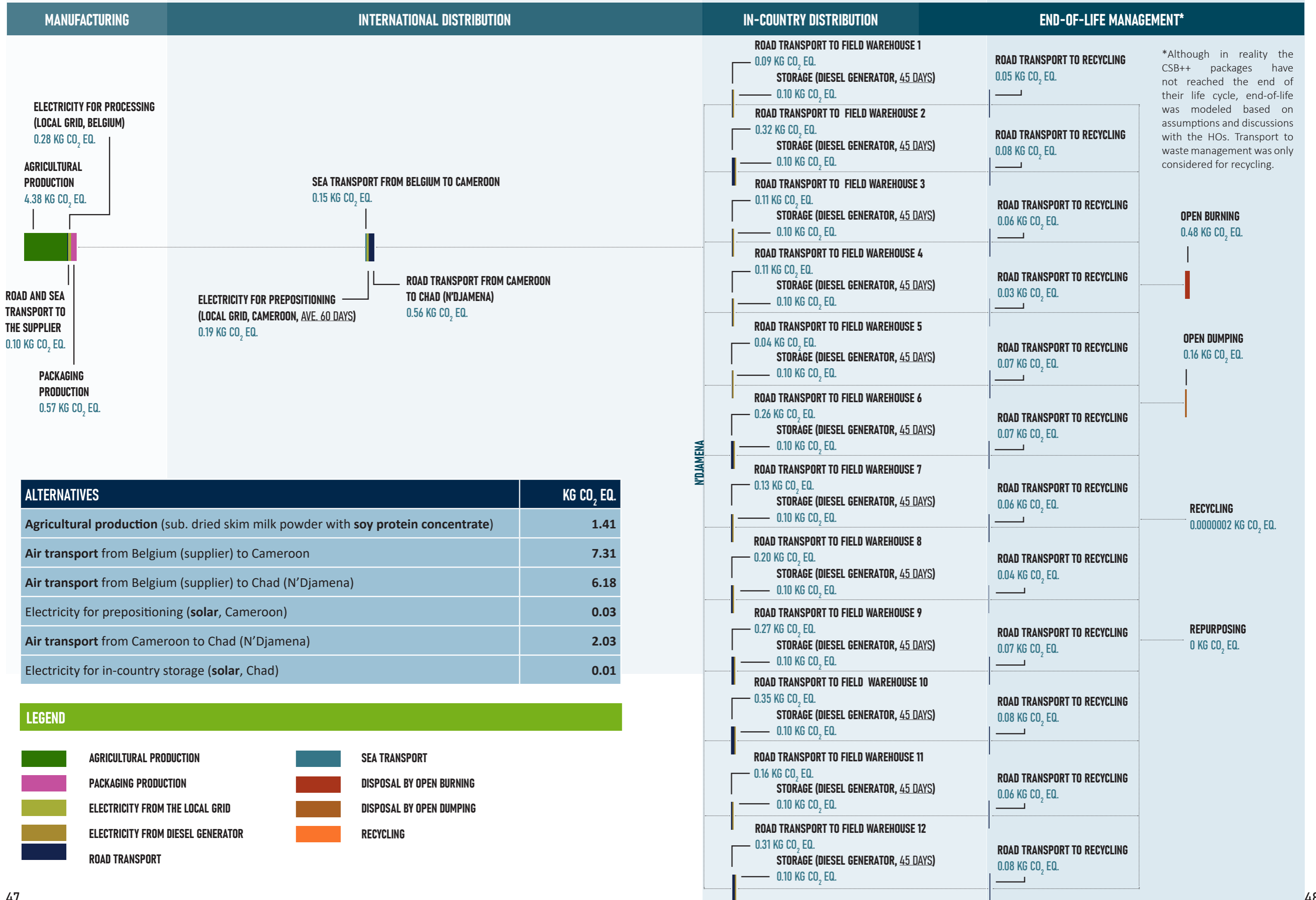
Fig. 14 Total GHG emissions for one unit CSB++ and packaging (total weight 1.72 kg) according to Case Study 3.
